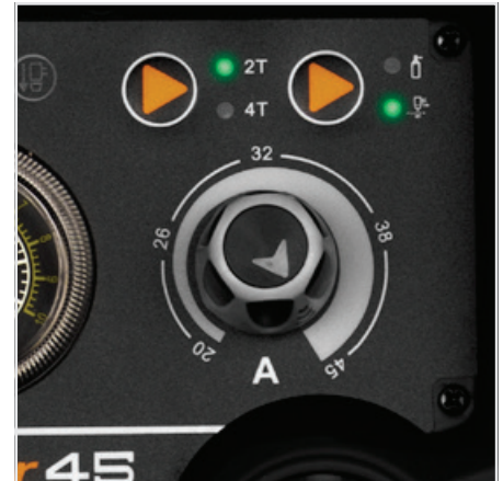
(5) Set 2T / 4T, then set the Amperage dial to the required setting.
